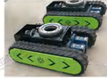
电动遥控底盘带回转 Electric remote-controlled tracked chassis with slewing function
