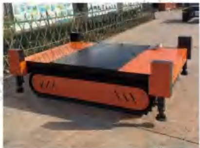
电动遥控履带底盘带液压支腿 Electric remote-controlled tracked chassis with hydraulic outriggers
