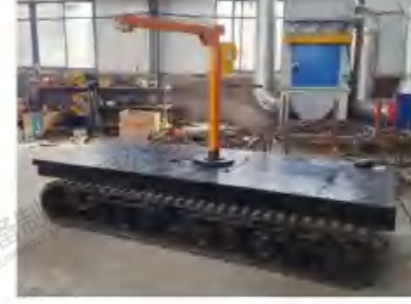
电动遥控履带底盘带吊臂 Electric remote-controlled tracked chassis with crane arm
